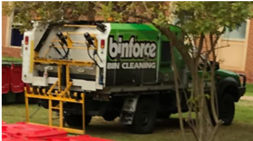
Figure 5-2: On-site bin wash system for rear-lift trucks on back of ute. Source: http://binforce.com.au/
