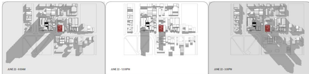
Figure 6 - shadow diagram during winter solstice.
