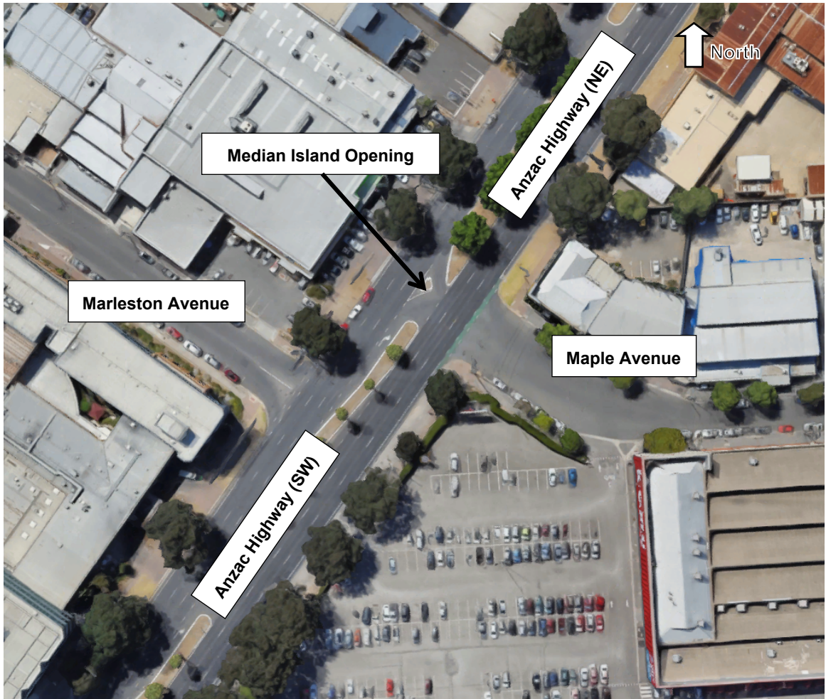
Figure 3: Junction layout- Maple Avenue/ Anzac Highway junction and Marlestone Ave/ Anzac Highway junction
