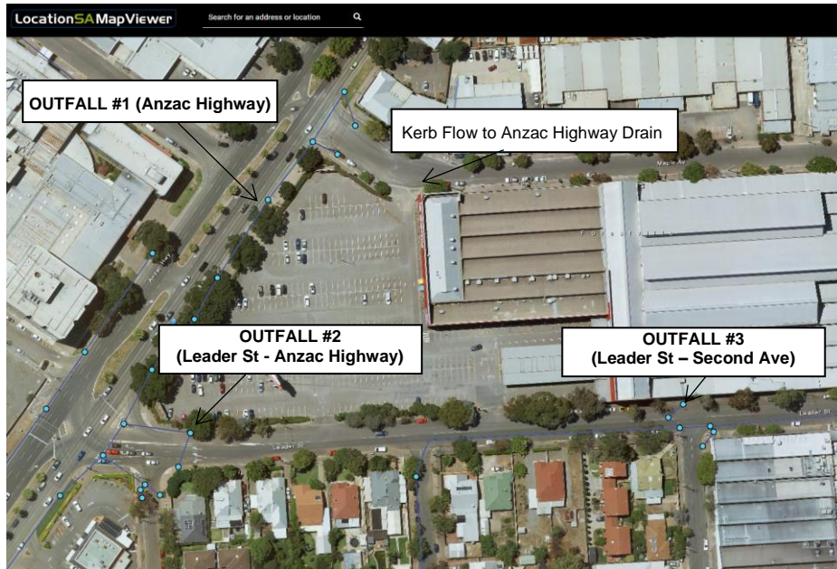
Figure 1 Existing drainage outfalls
