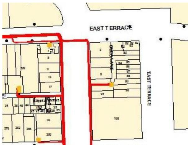
*Figure 1 - Details of existing SAPN High Voltage Infrastructure*
