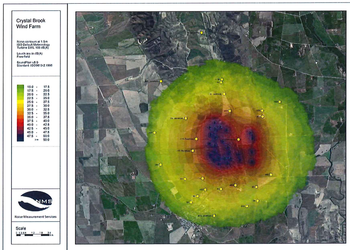
Plate 1: Calculations under ISO 9613-2 default settings, turbines at 105 dB(A) sound power level
