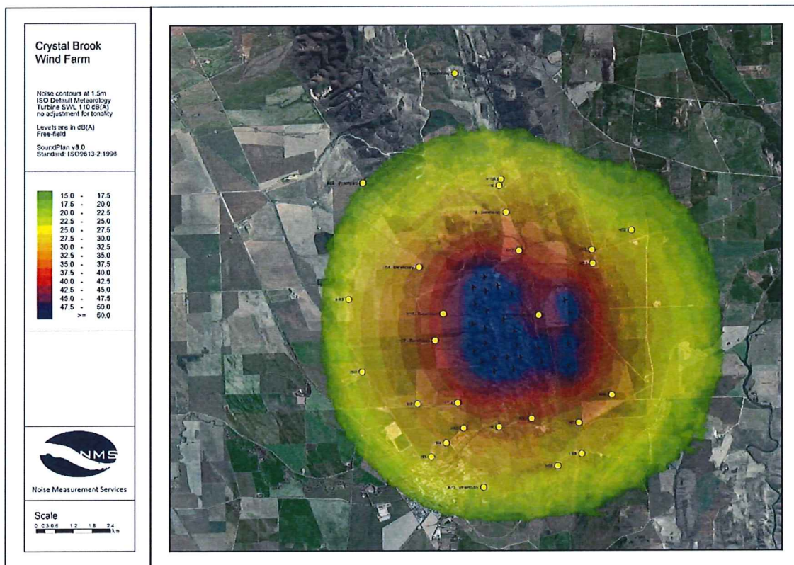
Plate 4: Calculations under ISO 9613-2 default settings, turbines at 110 dB(A) sound power level
