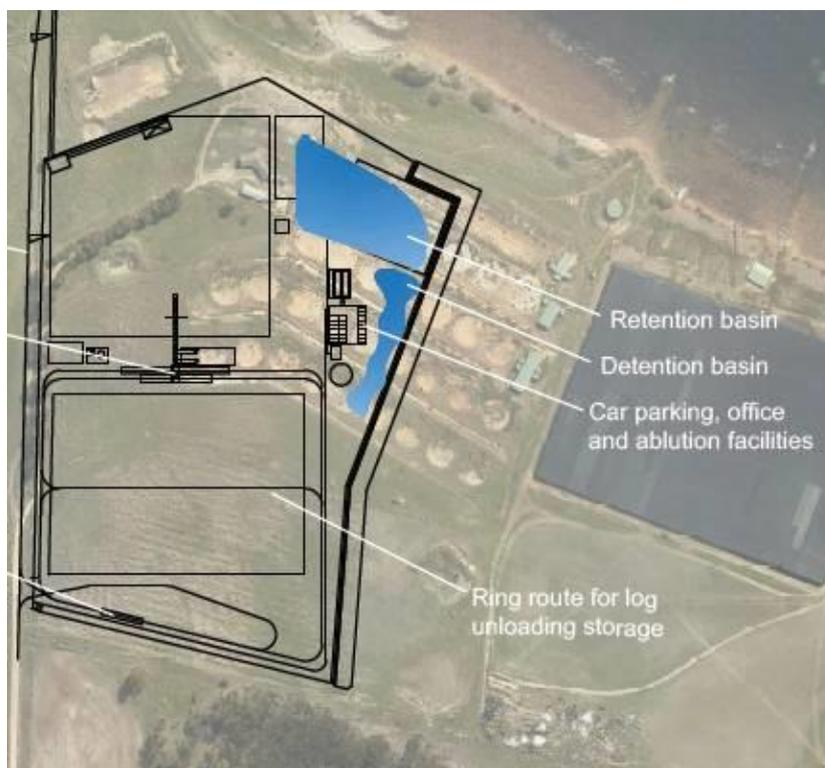
**Figure 40: Location of proposed ephemeral wetland (detention basin) and retention basin (EIS Figure 4-3)**
