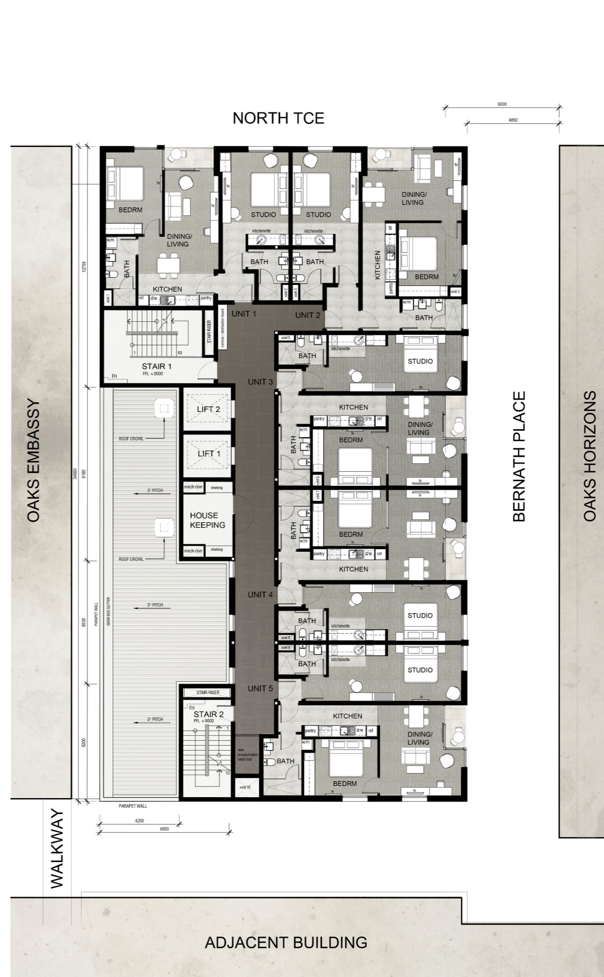
SECOND FLOOR PLAN PROPOSED PLAN SCALE: 1:100 GROSS FLOOR AREA: BUILDING - 550m 2 BALCONY - 12.1m 2
