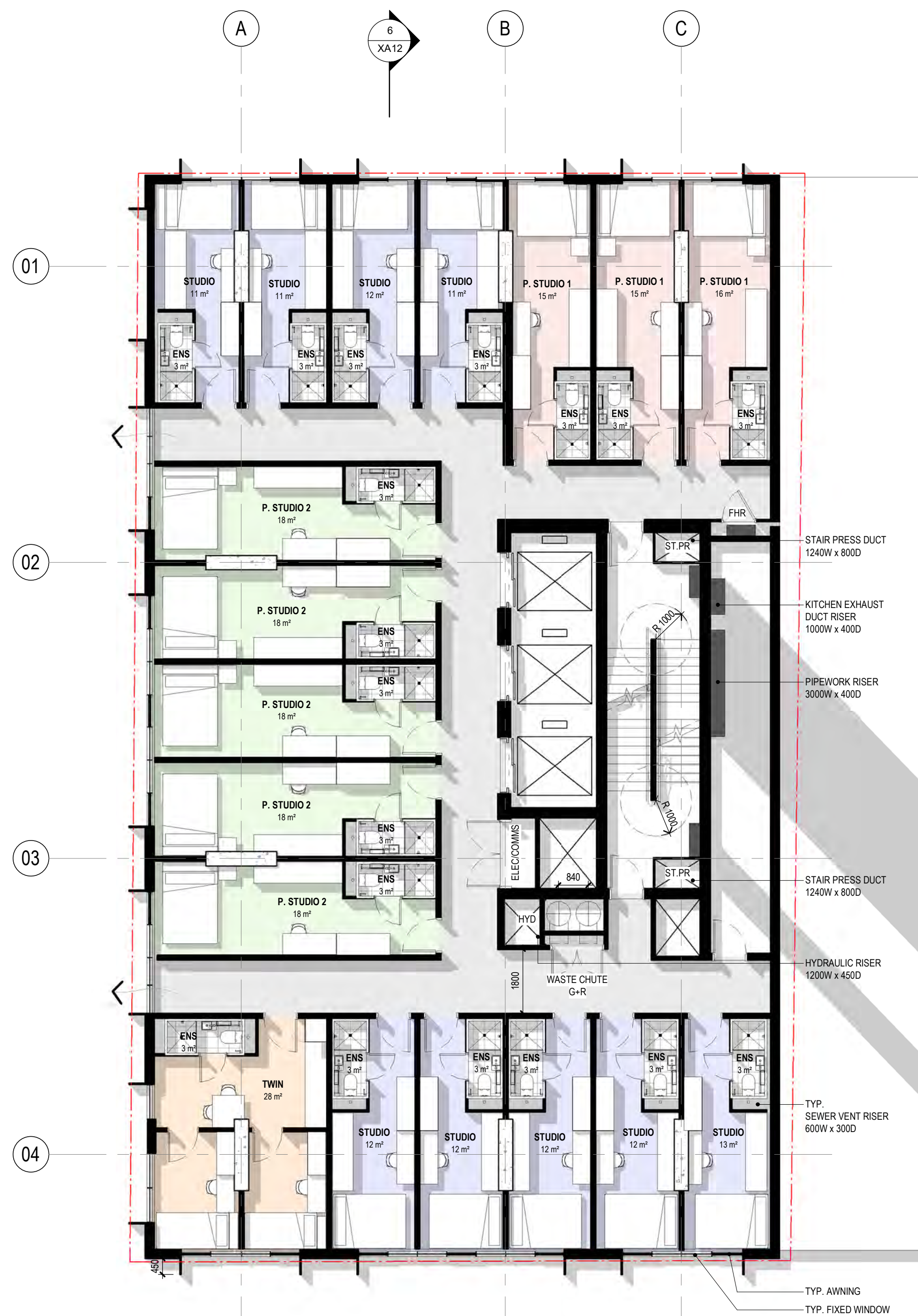
FLOOR PLAN, TYPICAL ARRANGEMENT- LEVEL 4-8 1 : 100
