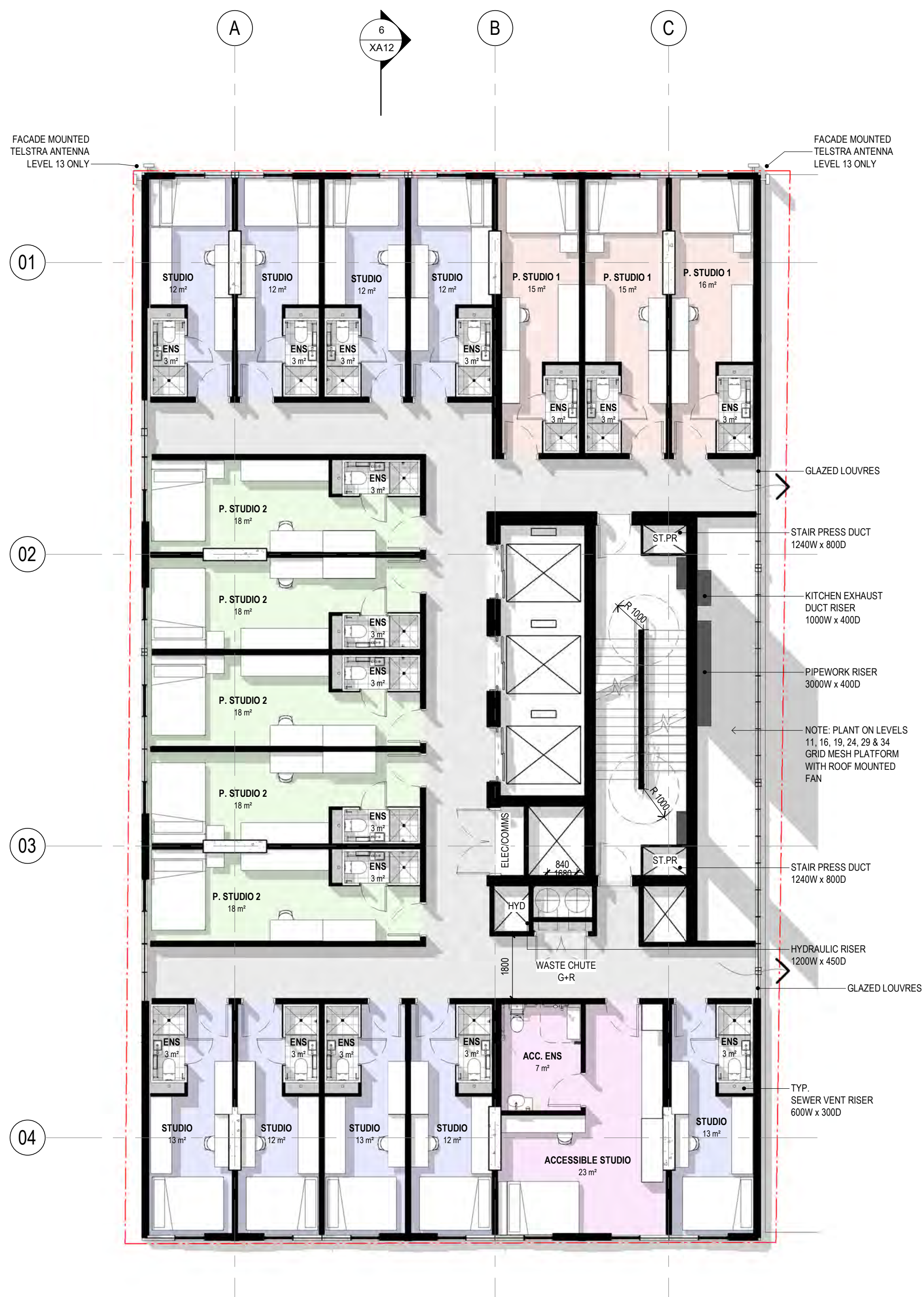
FLOOR PLAN, TYPICAL ARRANGEMENT - ACC.STUDIO + STUDIO 1 : 100
