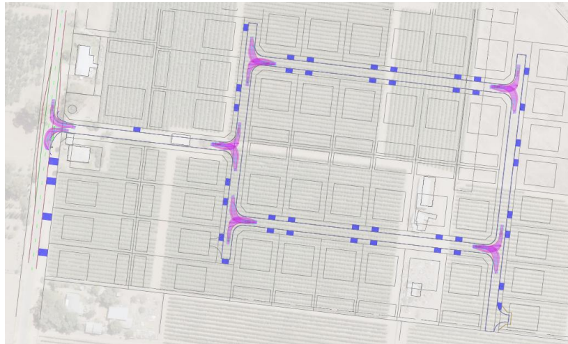
Figure 5: 12.5m heavy rigid vehicle turn paths (part of Cirqa dwg 26042 Sheet #01_SH02)
