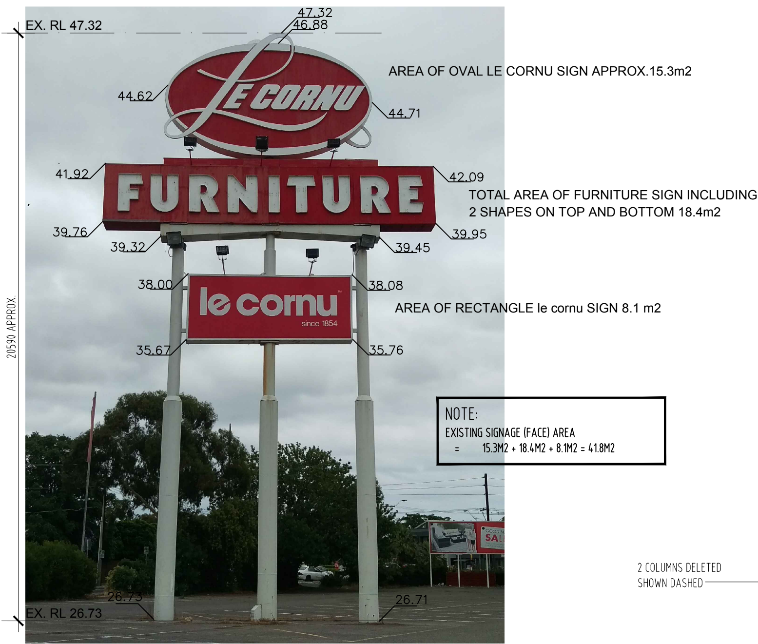
01 Existing Pylon Sign TP-02 Existing Elevation SCALE NTS (Survey from Alexander Symonds)
