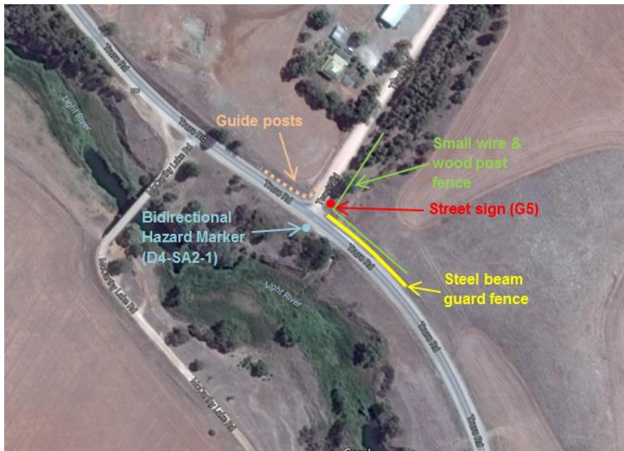
Figure 24 Street furniture located on A2I01/B2I01 (Truro Road / Teagle Road)
