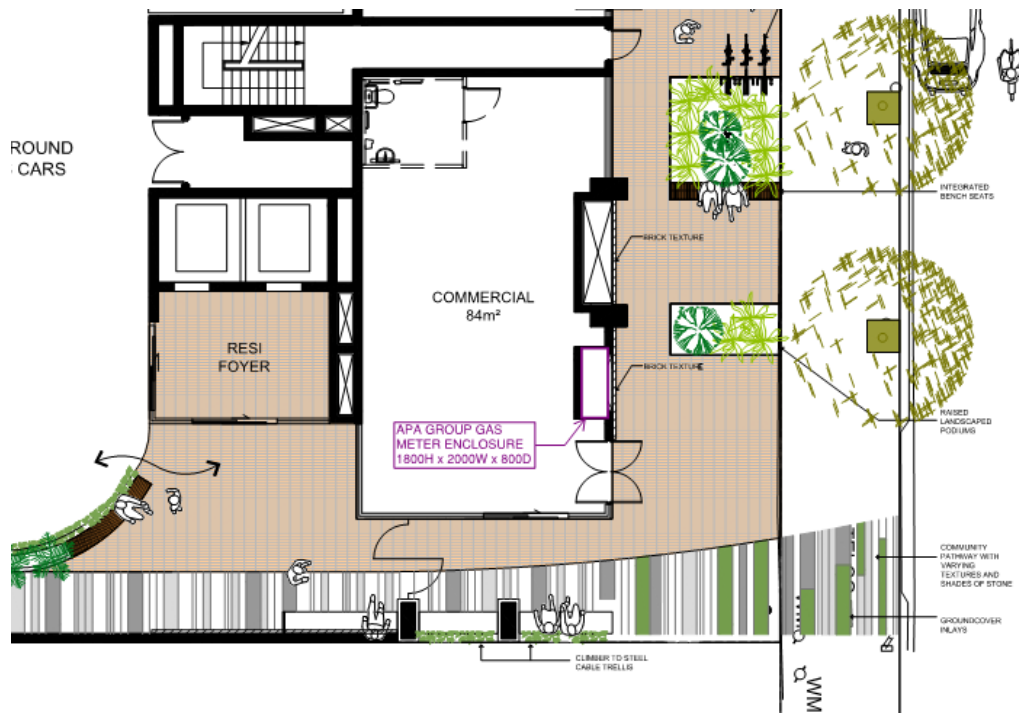
Figure 6: Proposed APA Group Gas Meter Enclosure Location
