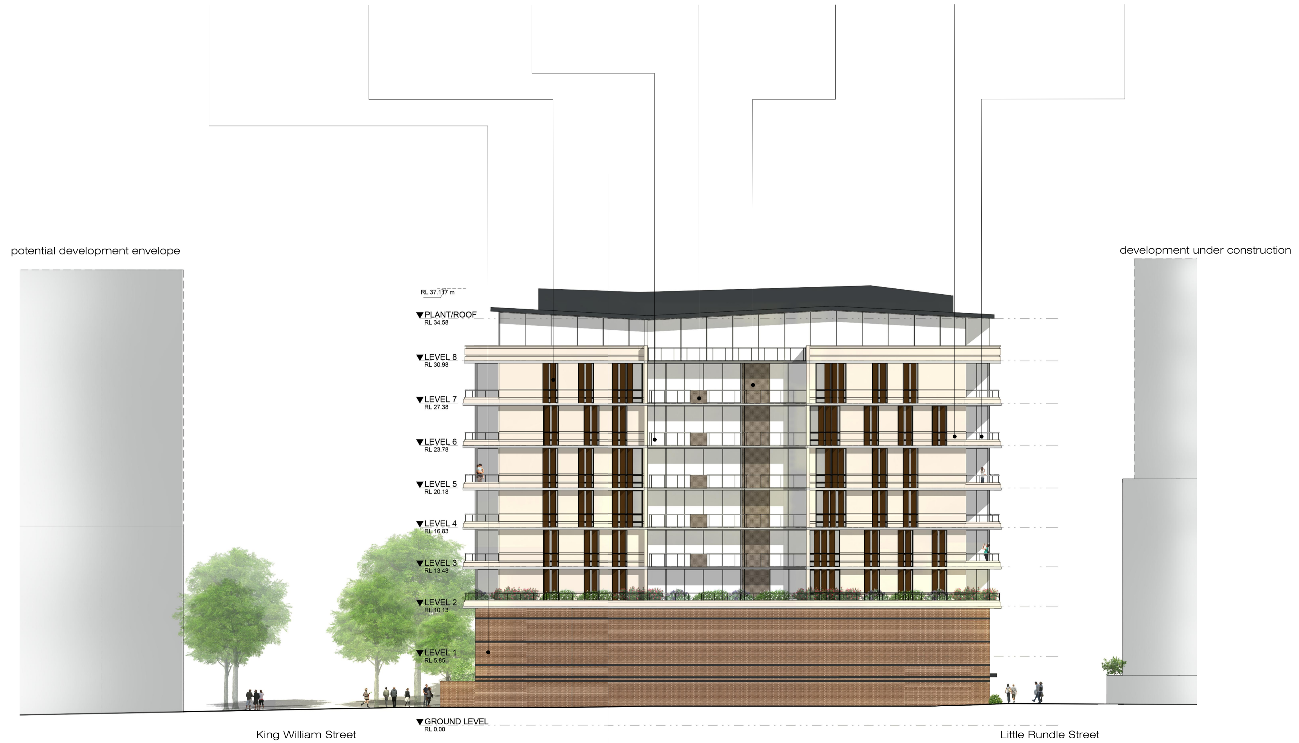
polished and textured precast concrete with horizontal recessed detailing
