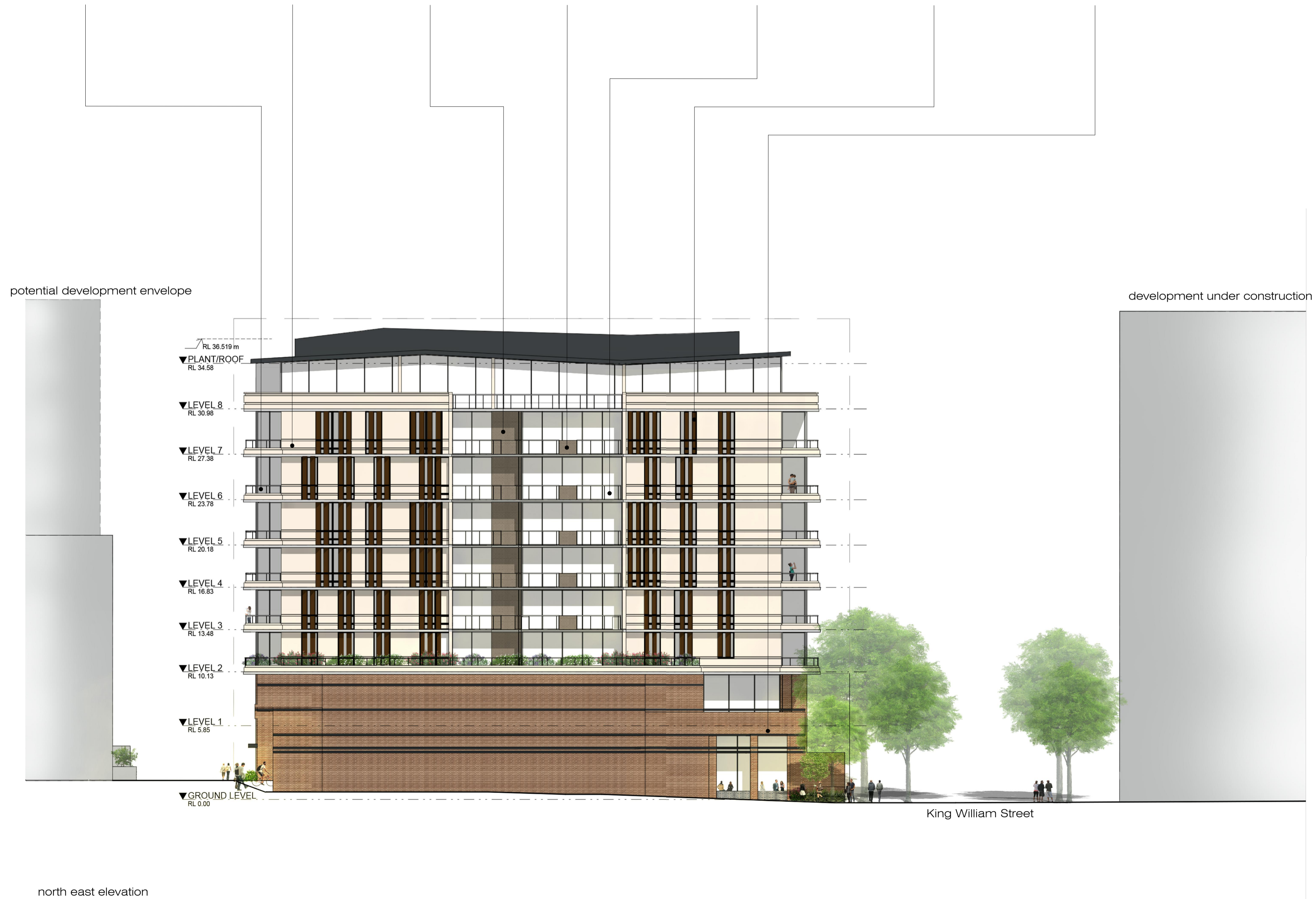
polished and textured precast concrete with horizontal recessed detailing
