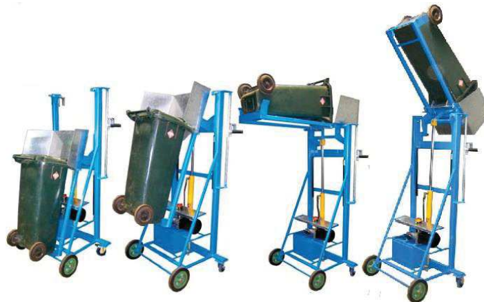
Figure 4-5 – Typical Mobile Garbage Bin lifter shown without protective cage (source: www.rjcox.com.au )
