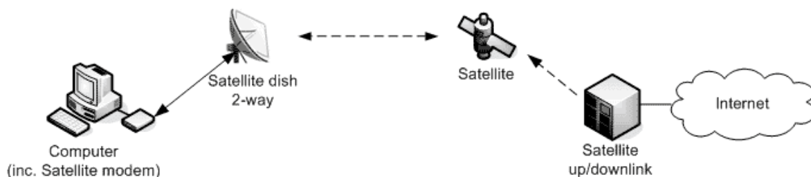
Two-way connection to the internet via satellite [24]
