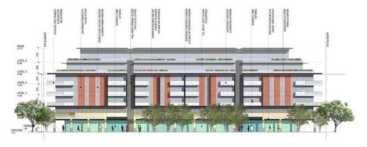
Figure 2.2 Side elevation and 30 degree building envelope
