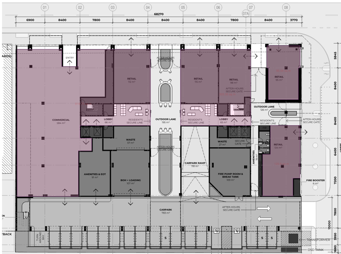
Figure 1 Highlighted Thermal Envelope of Ground Floor
