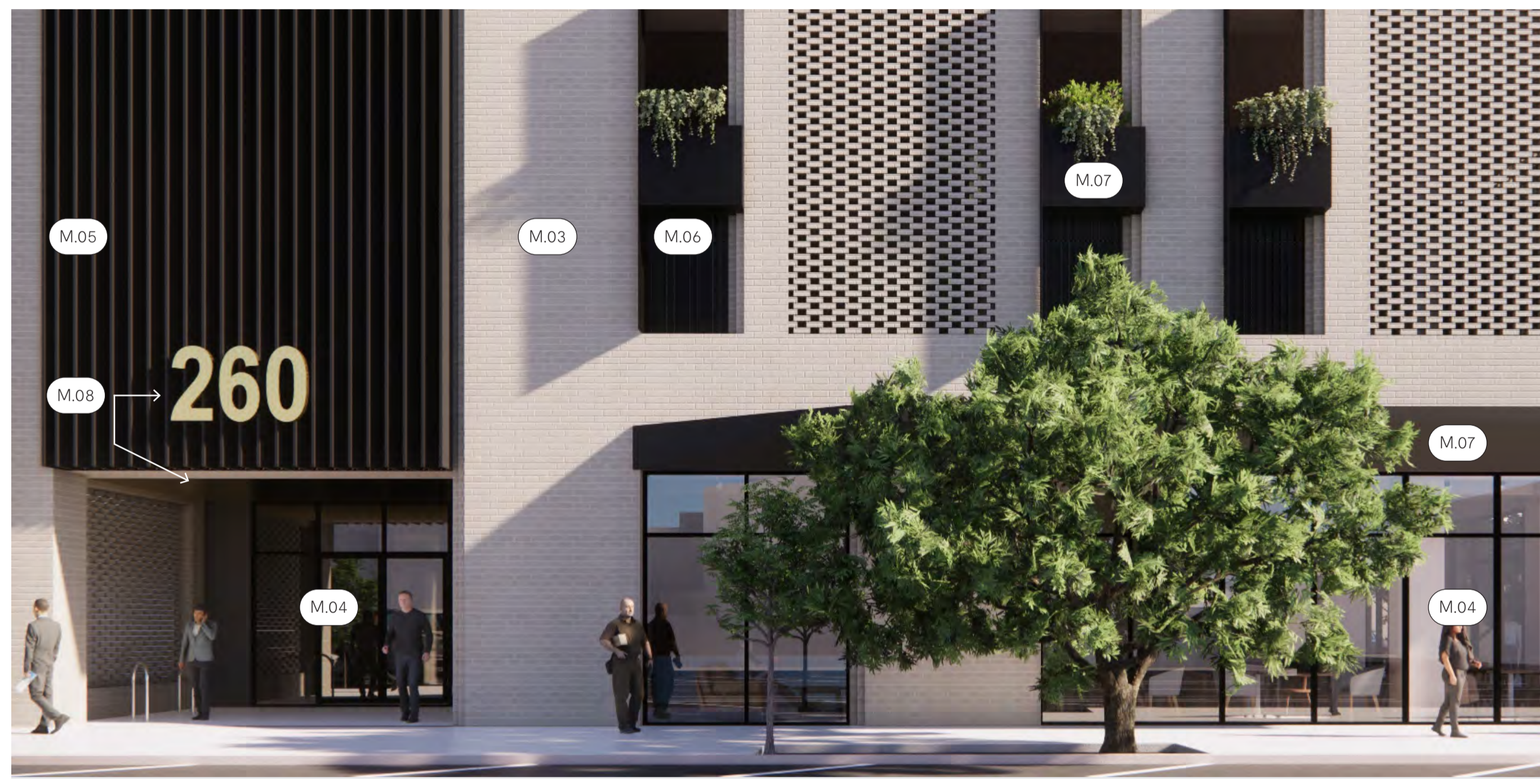
South Facade Detail Materials - Up close texture and detail where people can interact
