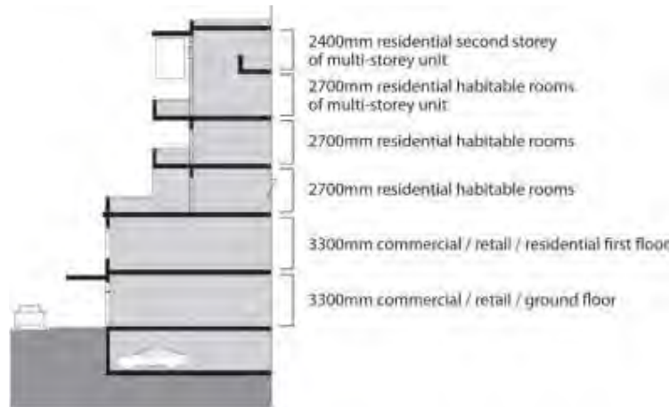
Figure 52.1 - appropriate ceiling heights for mixed use buildings.
