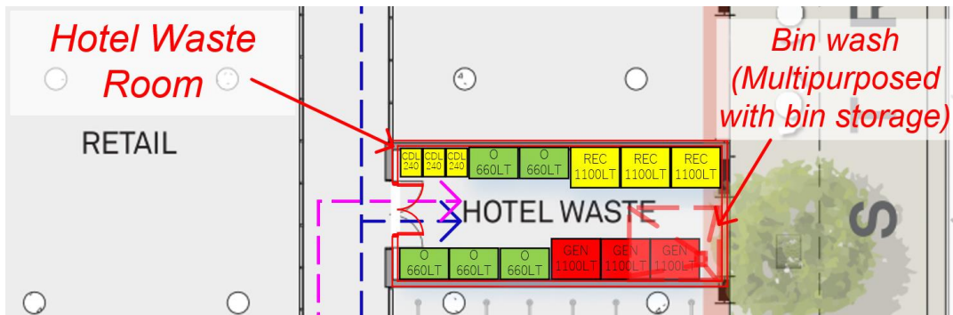
Figure 3-2: Detailed view of Hotel Waste Storage Room. Note: Bin labels are: G – General Waste; R – Recycling; O – Organics, CDL – Container Deposit
