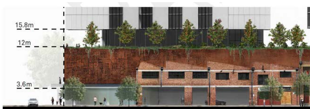
Figure 23 – Incorporation of existing masonry façade and proposed façade Source: Hassell
