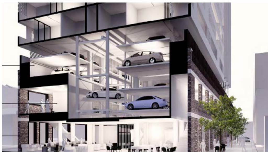
Figure 14 – Section illustrating concealed car stacking system Source: Hassell
