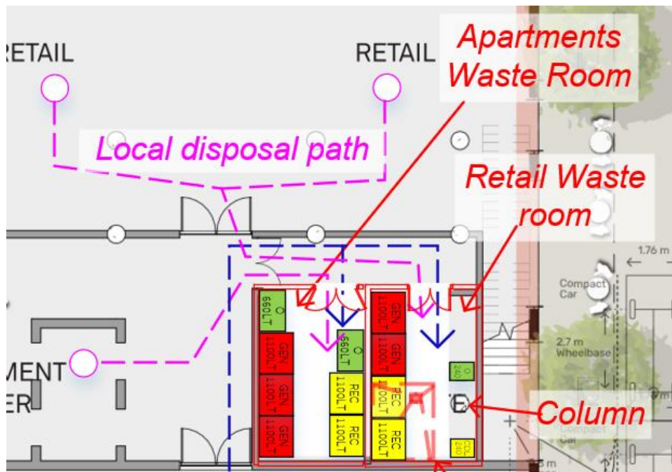
Figure 3-3: Detailed view of Apartments and Retail Waste Storage Rooms. Note: Bin labels are: G – General Waste; R – Recycling; O – Organics, CDL – Container Deposit
