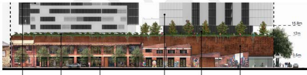
Figure 13 – Existing masonry facades to be incorporated into podium Source: Hassell
