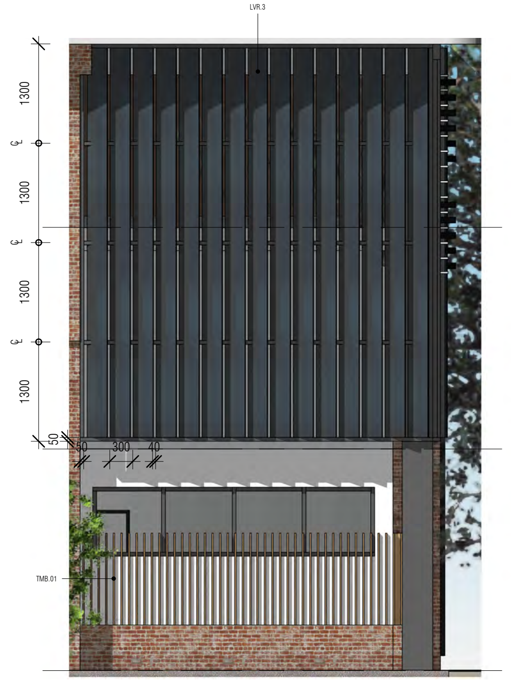
3 WEST ELEVATION - LOUVRE 3 DETAIL DA53 1:50
