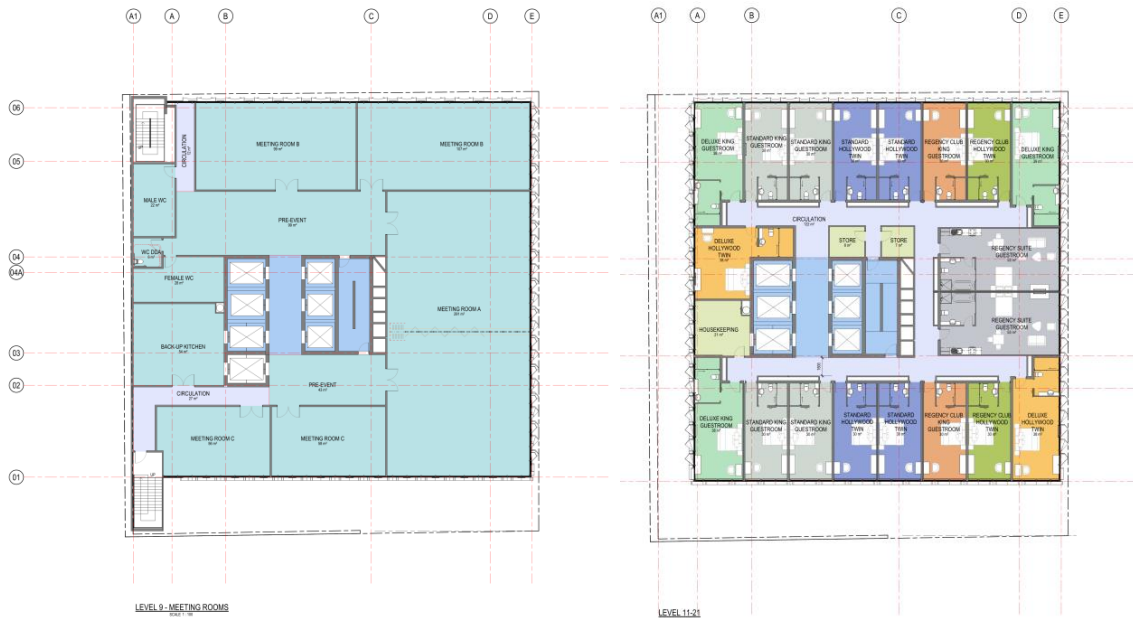
Figure 3: The building's footprint remains consistent on the majority of floors, resulting in minimal exposed floors and ceilings throughout the building.
