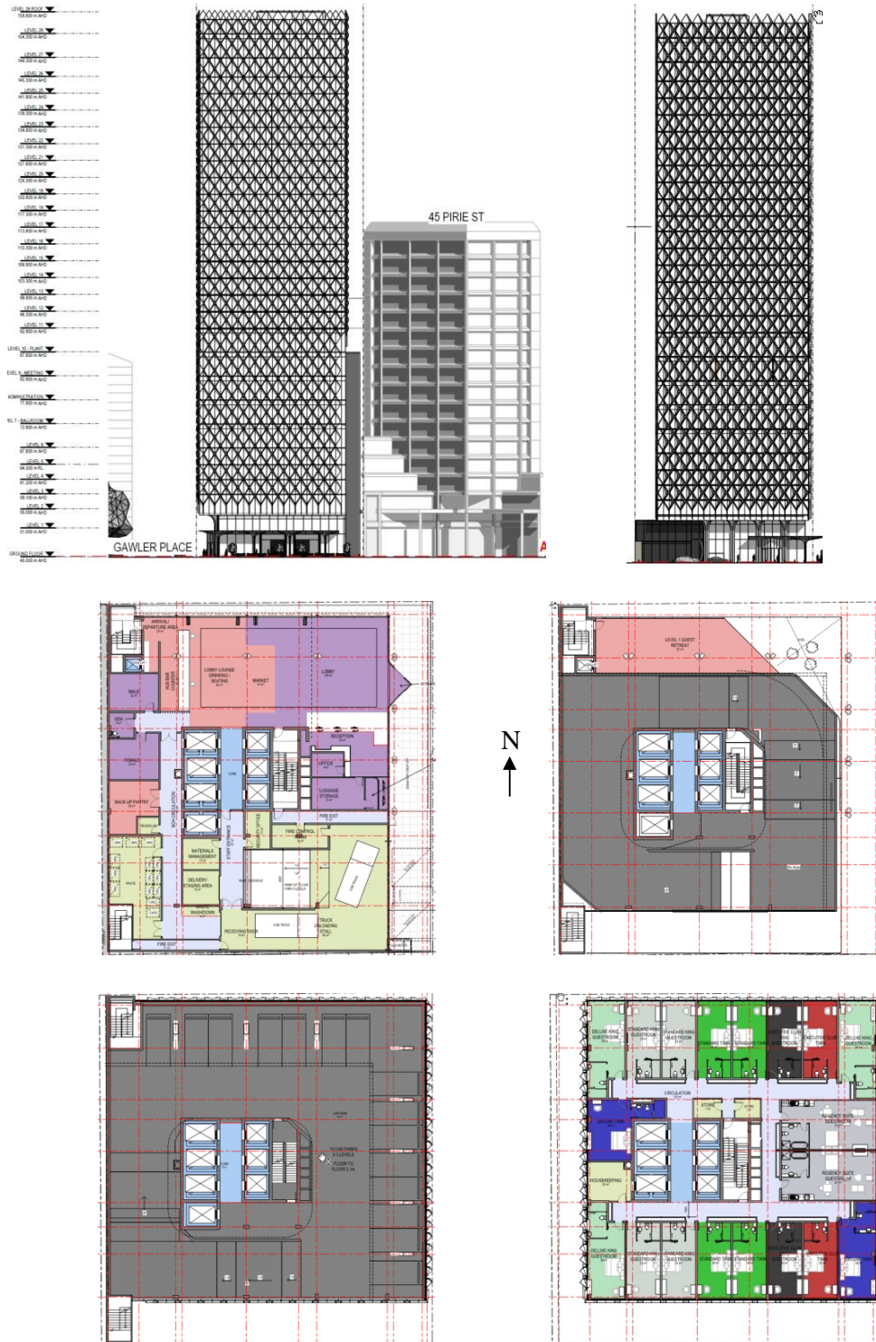
Figure 2: North elevation (TL), East elevation (TR), and Floor plans: Ground floor (ML), Level 1 (MR), Level 2 (BL), and Levels 11-21 (BR).
