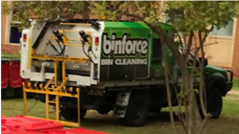
Figure 4-3 – On-site bin wash system for rear-lift trucks on back of ute. Source: http://binforce.com.au/
