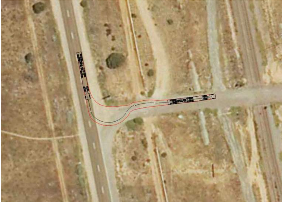
Figure 4-12 - B-Double accessing Lincoln Highway Access Point
