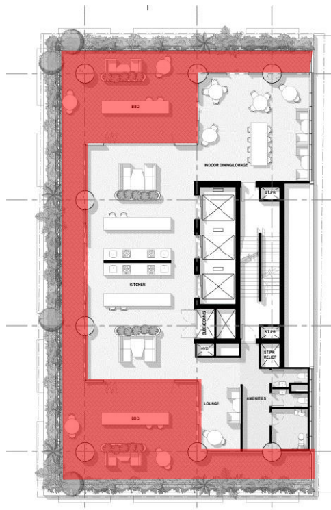
Figure 7: Ground floor with recommended wind criteria overlaid.
