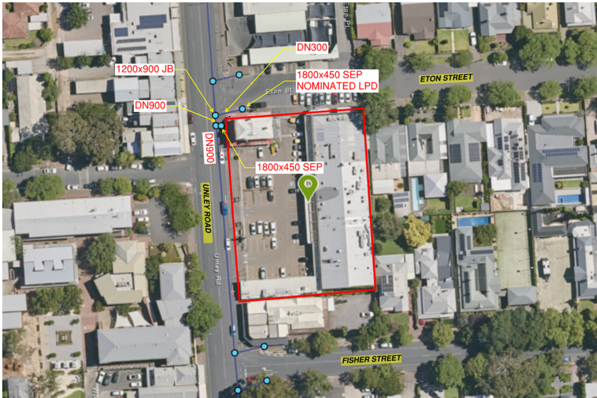
Fig.02 – Adjacent Stormwater Infrastructure
