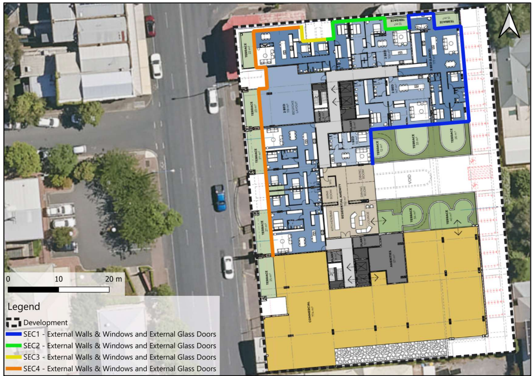
Figure 4 Extent of MBS 010 treatment on Level 1
