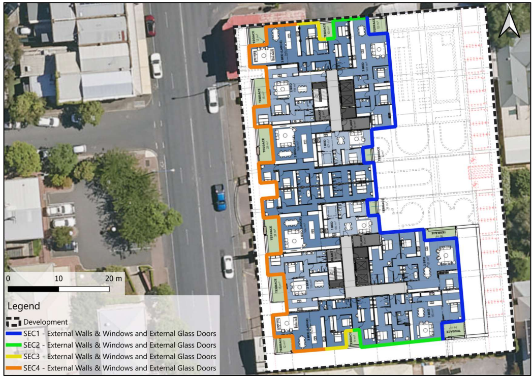
Figure 7 Extent of MBS 010 treatment on Level 4
