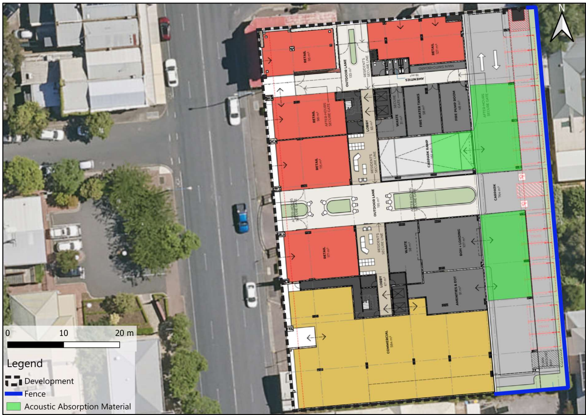
Figure 12 Noise Control Measures
