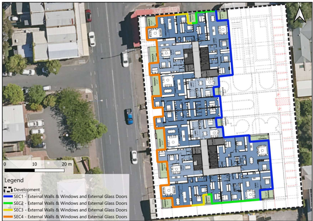
Figure 8 Extent of MBS 010 treatment on Level 5
