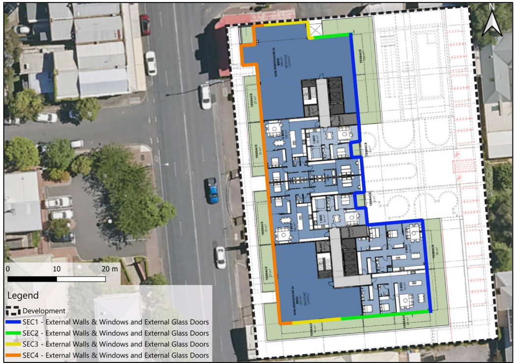
Figure 9 Extent of MBS 010 treatment on Level 6
