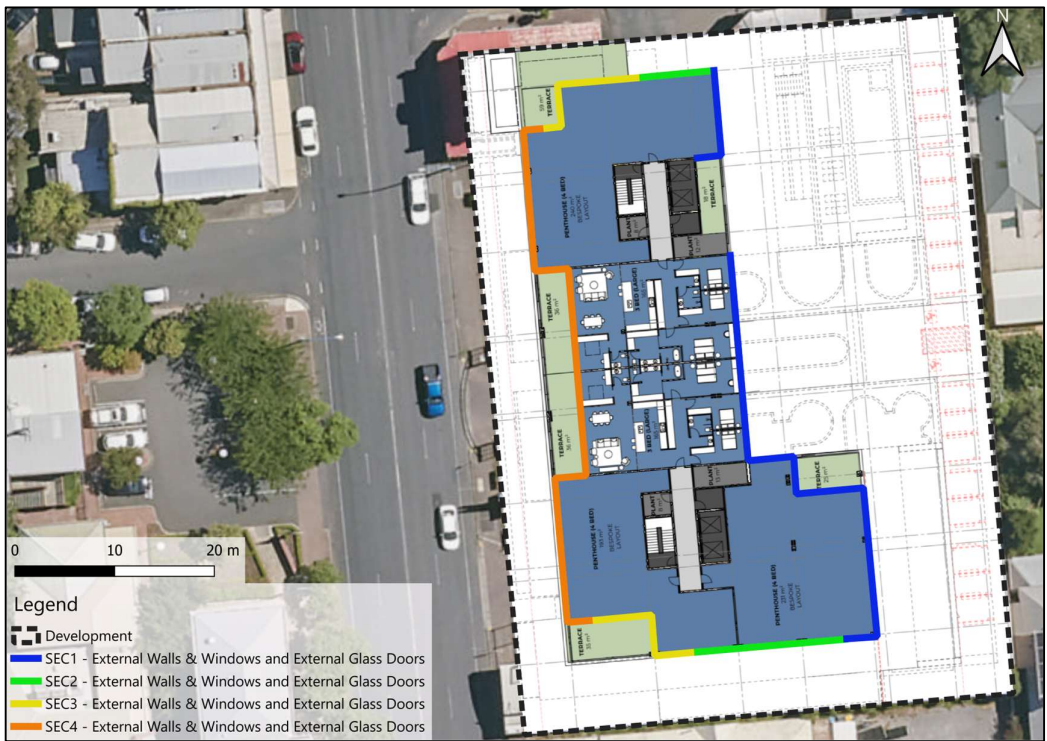
Figure 10 Extent of MBS 010 treatment on Level 7
