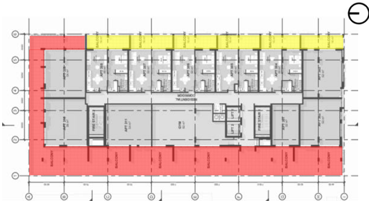
Figure 7: Ground floor with recommended wind criteria overlaid
