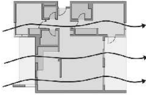
Figure 58.2 - optimal layout allowing air flow directly from one side of a dwelling/apartment to the other.
