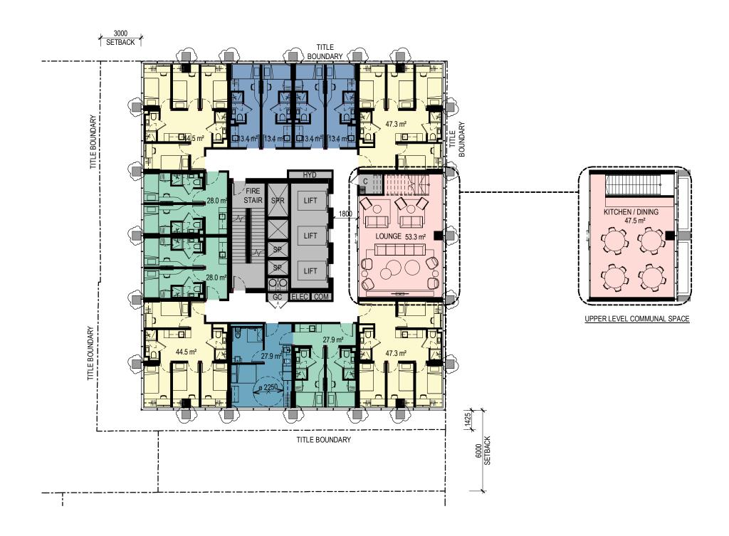
CLEANERS CUPBOARD COM COMMUNICATIONS RISER ELEC ELECTRICAL RISER GC GARBAGE CHUTES HYD HYDRAULICS RISER
