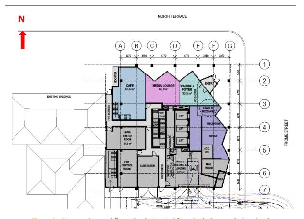
Figure 4 – Proposed ground floor plan (extracted from Rothelowman's drawings)
