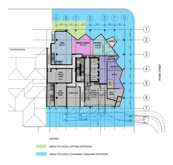
Figure 13 – Ground floor plan with recommended criteria overlaid
