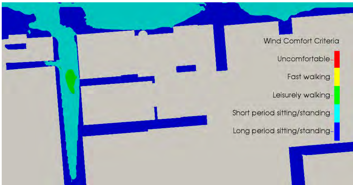
Figure 16: Pedestrian level wind comfort assessment contours for the existing buildings, viewed from above.
