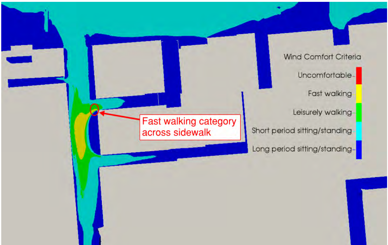
Figure 19: Pedestrian level wind comfort assessment contours for the proposed development, viewed from above.
