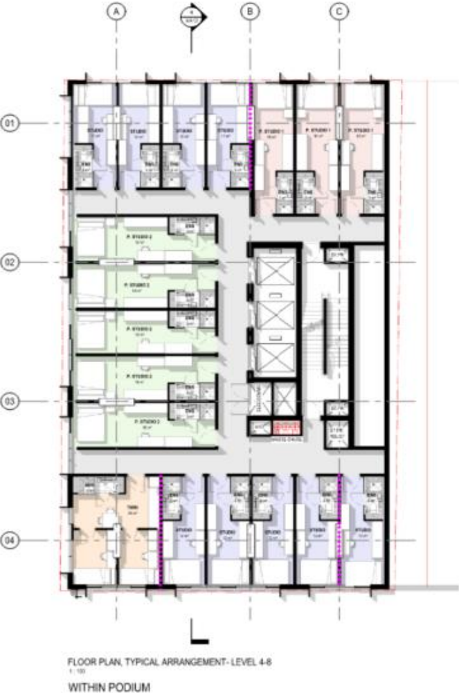
Figure A 5: Level 4-8 Discontinuous Construction Markup
