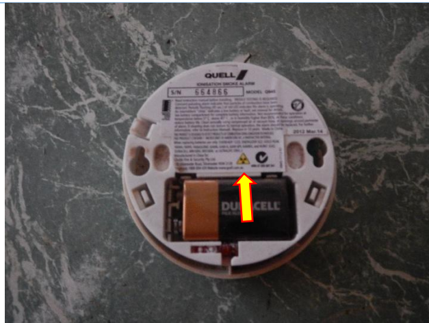
Smoke detector identifies radioactive isotope
