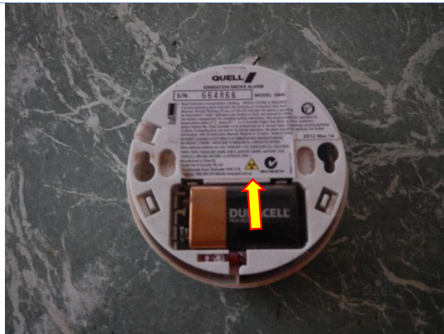
Smoke detector identifies radioactive isotope
