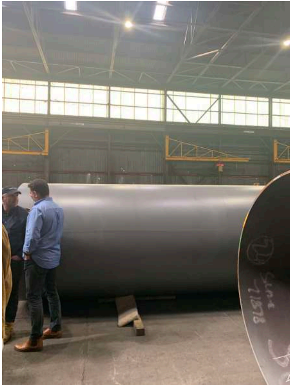
1 Elizabeth Steelwork welding for Concrete-filled columns - Round 1 - May 2021
