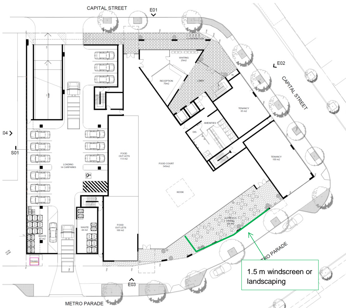
Figure 7: Schematic plan view of the ground floor with recommended wind control measures
