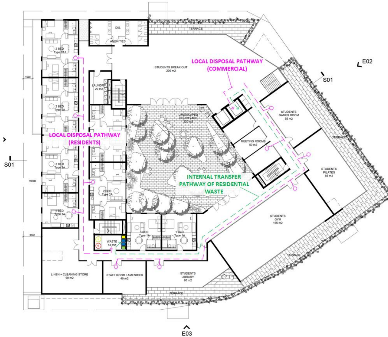
Figure 5-2: Level 1 layout showing disposal paths and waste room. Yellow = 140L CDL Bin, Blue = 140L Bulky cardboard bin, Green = Organics/Food Waste
