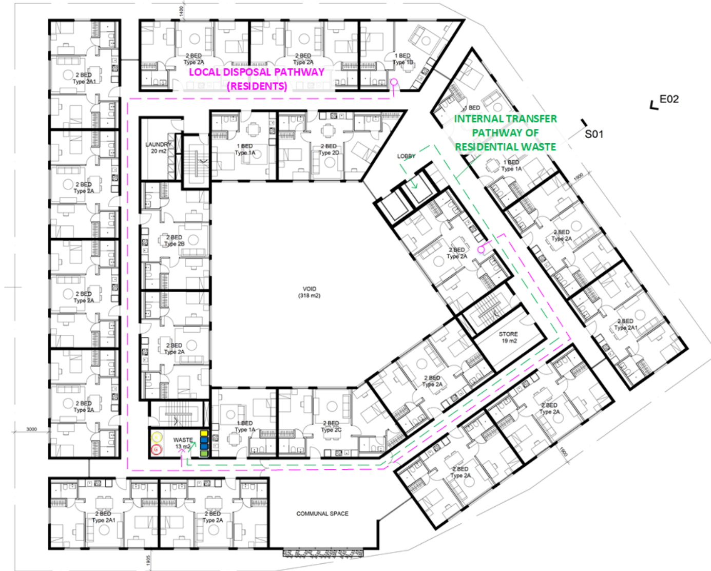
Figure 5-3: Typical Apartment level layout showing disposal paths and waste room. Yellow = 140L CDL Bin, Blue = 140L Bulky cardboard bin, Green = Organics/Food Waste.
