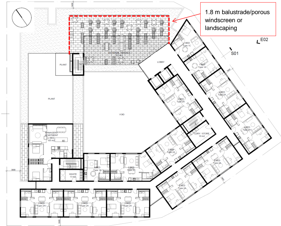
Figure 8: Schematic plan view of the roof terrace with recommended wind control measures
