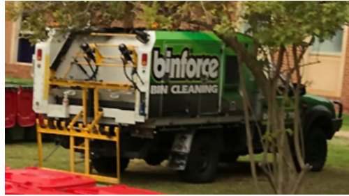
Figure 3 – On-site bin wash system for rear-lift trucks on back of ute. Source: http://binforce.com.au/
