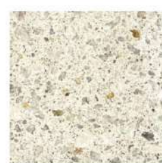
PC1 DECORATIVE PRECAST CONCRETE EXPOSED AGGREGATE
