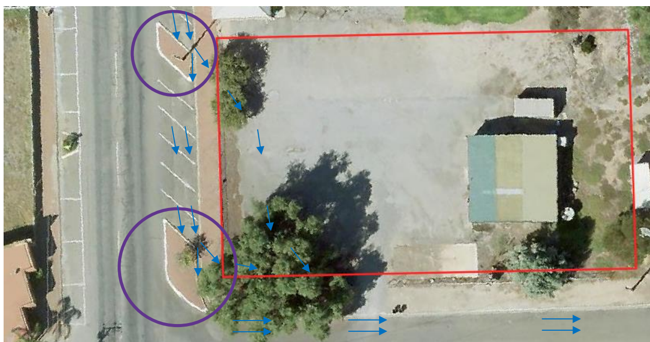
Figure 4.1 - Disconnected protuberances along Old Port Wakefield Road and expected flow paths for gutter flow spill
