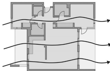
Figure 58.2 - optimal layout allowing air flow directly from one side of a dwelling/apartment to the other.
