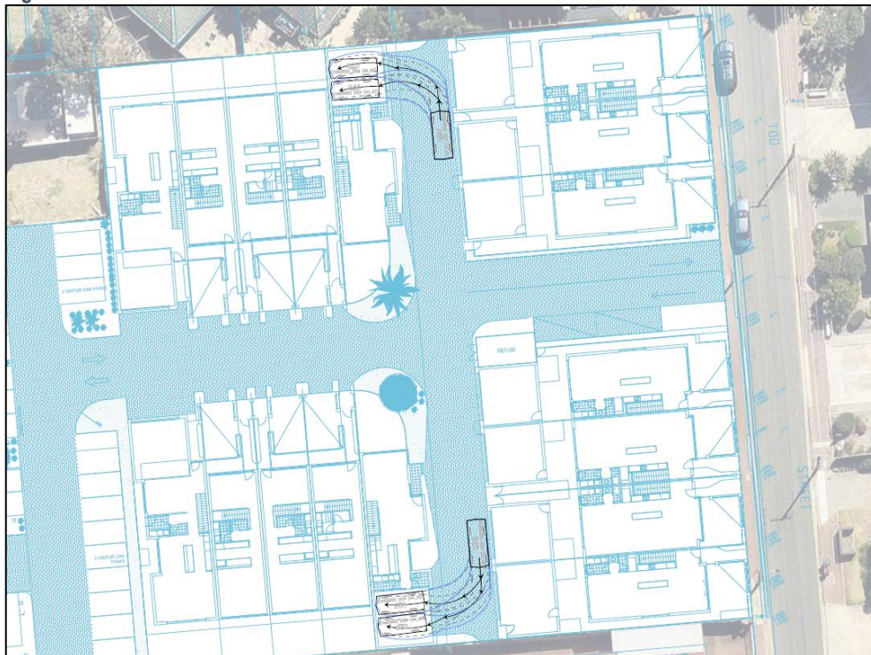
Figure 4.1: Blind aisle extensions with B85 reverse movement
