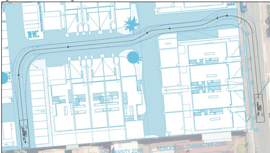
Figure 6.1: 8.8m MRV entering the site in a forward direction
