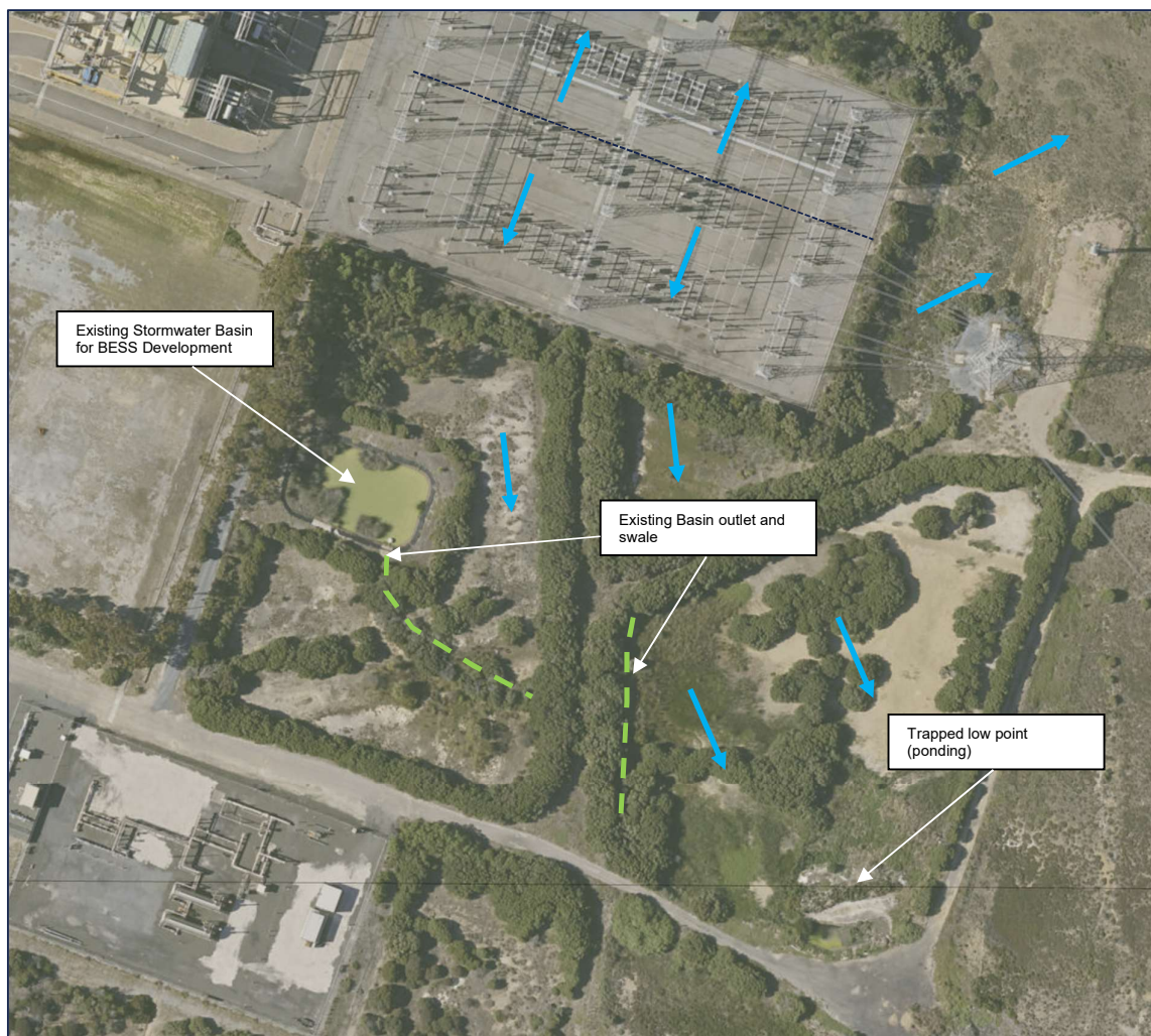
Figure 4 Existing Stormwater Infrastructure
